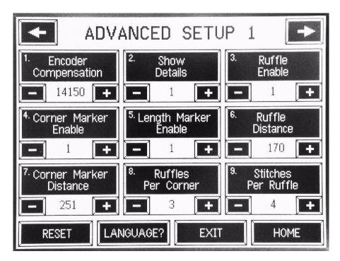
This screen displays the internal machine settings that control all functions. The number in the upper left corner of each button represents the counter/setting number and is used on the SHOW ALL SETTINGS page matrix. Notice that the RUFFLE ENABLE setting is the same setting as the RUFFLE ENABLE button on SETUP BORDER MODE page 2 mentioned earlier. The same is true for many of the other settings shown.
