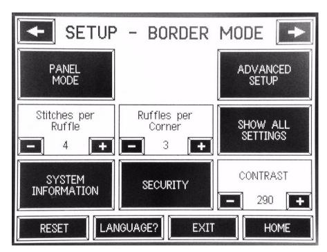
This allows setup of the ruffle quantity and stitches, access to SECURITY, SYSTEM INFORMATION, ADVANCED SETUP, and the SHOW ALL SETTINGS matrix screen. The CONTRAST button changes the screen contrast. The "+" and "-" buttons change the counters.
