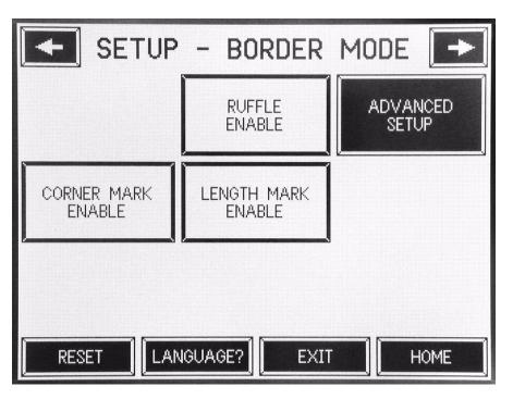
Note: when a button has a white background the function is on or enabled. A dark background indicates off or disabled. Press the top arrows to return to the first SETUP screen.
