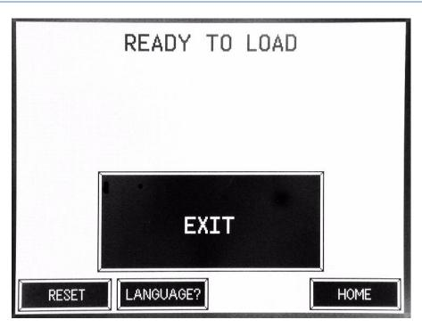
Press EXIT to lower the foot, etc., and return to the main screen. The HOME button takes you to the main screen without resetting the machine.
